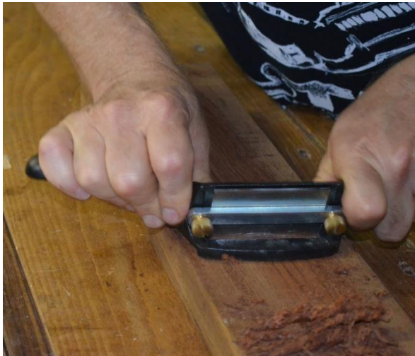
Demonstrating the use of a Stanley Scrapper Plane which has many advantages for large surfaces.
