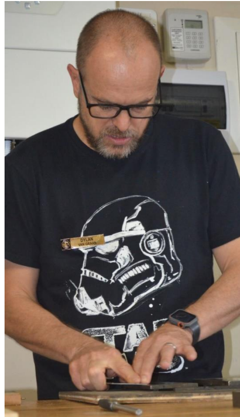
The two side faces of the scraper are first prepared. Only about 3-5 mm width needs attention.
