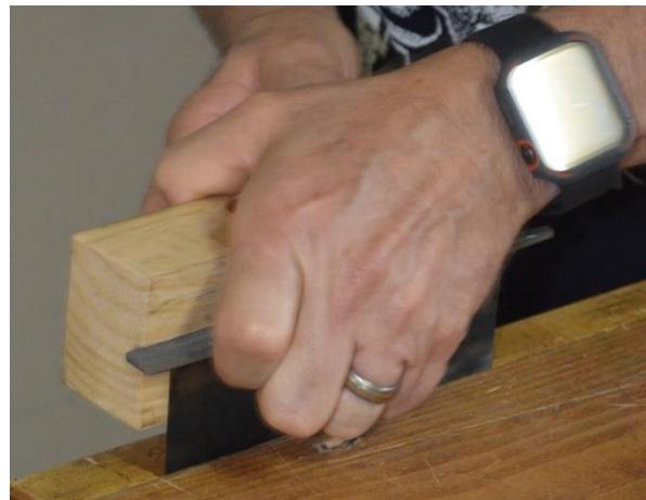
The edge is then filed down using a 2 nd cut file mounted squarely in a wooden block. The scraper is clamped in a vice and the filing continues until there is equal resistance along the full length. Remove the burr on the sides on the fine stone.
