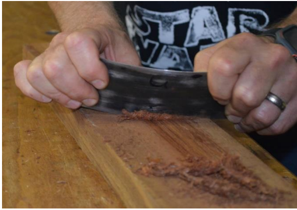
Testing the newly sharpened scraper on kiaat. Note the fine shavings.
