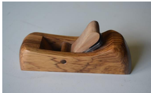
Paul Roberts showed this small block plane made in ironwood equipped with a Ron Hock blade and chip breaker.
