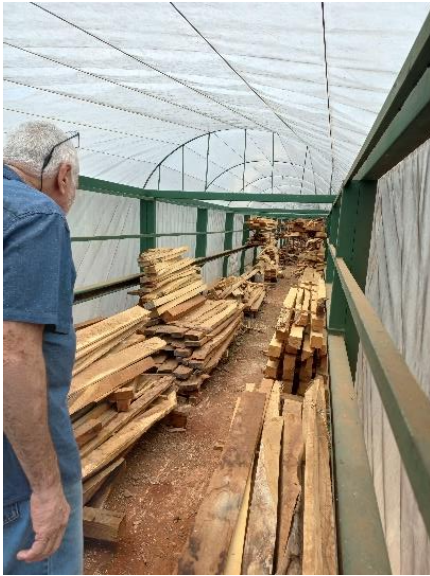
Wood being cured in the tunnel.
