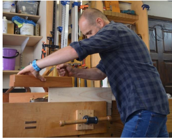
Planing action using your legs for thrust.
