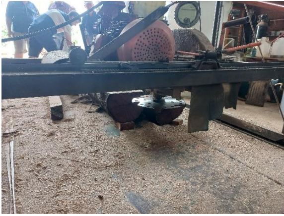
Saw blade in the horizontal position.
