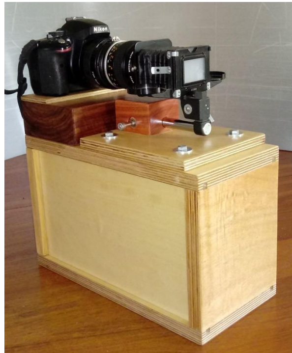
Paul Roberts developed and made this slide copying system. The mounting box is made from birch plywood.
