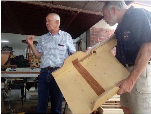
Willie Marneweck explaining details of his cross cut sled for his table saw.
