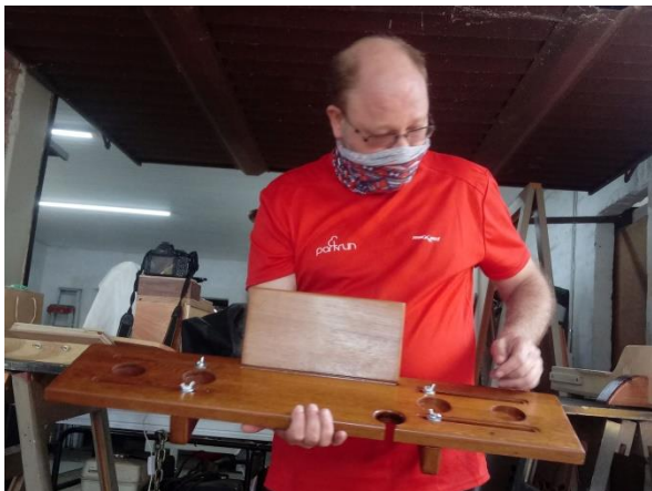
Pieter Vrolijk made this bath caddy, with space for four tealight candles, a wine glass and a tablet/cellphone. It has adjustable stays underneath to make sure it doesn't slip sideways while in use. Made from red alder.
