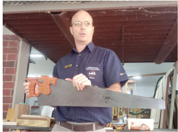
Corneel du Toit renovated this handsaw. He made a new handle and had to import the saw nuts from the USA.
