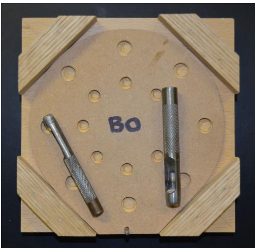
Willie Marneweck prepares his own circular sanding discs using a template and punches.
