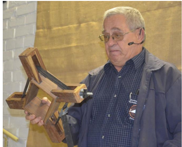
Leon Wolamarans with the shop-made strap clamps he made for small wooden boxes.
