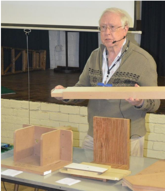
Paul Roberts illustrating the table saw jig he made for cutting tenons on a table saw.
