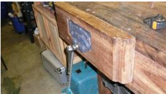
A photo showing the wooden jaw that Ben added to the metal jaw of his vice
