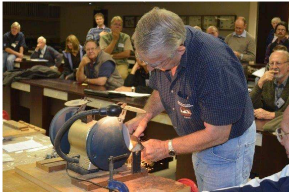
Bevel grinding on a chisel
