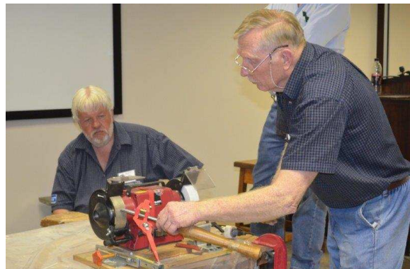
Sharpening a bowl gouge using a jig
