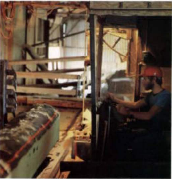
The headsaw, a 150-HP bandsaw, can slice the length of a 16-ft. log in less than two seconds. Here the log is being manipulated for a second cut; the red line is a laser beam that shows the sawyer where the cut will be.
