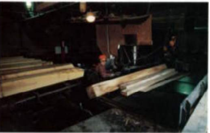
Squared-up logs, called cants, are sawn into boards on a bandsaw similar to the head rig shown above and on p. 40. Here the sawyer has just seen a defect in the cant, and is flipping it to a new, clean face for the next cut.
