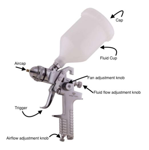
The gun consists of an aluminium body, equipped with a plastic or aluminium cup and a cap for the paint. The paint can flow under gravity down to the nozzle (usually with an orifice of 1.4mm diameter). The orifice of the nozzle is kept closed by a spring-loaded needle. The latter may be pulled back, opening the orifice, by means of a trigger.
