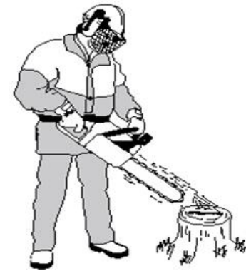
Check Oil Pump
