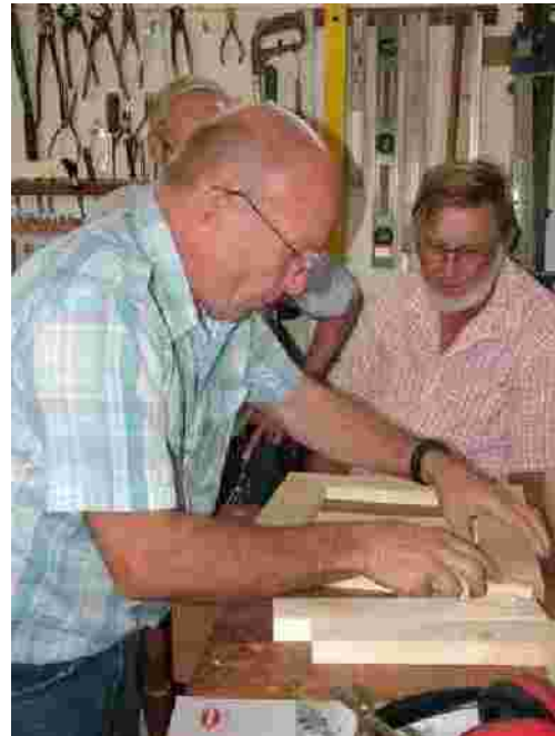
Dry assembly of the frame components
