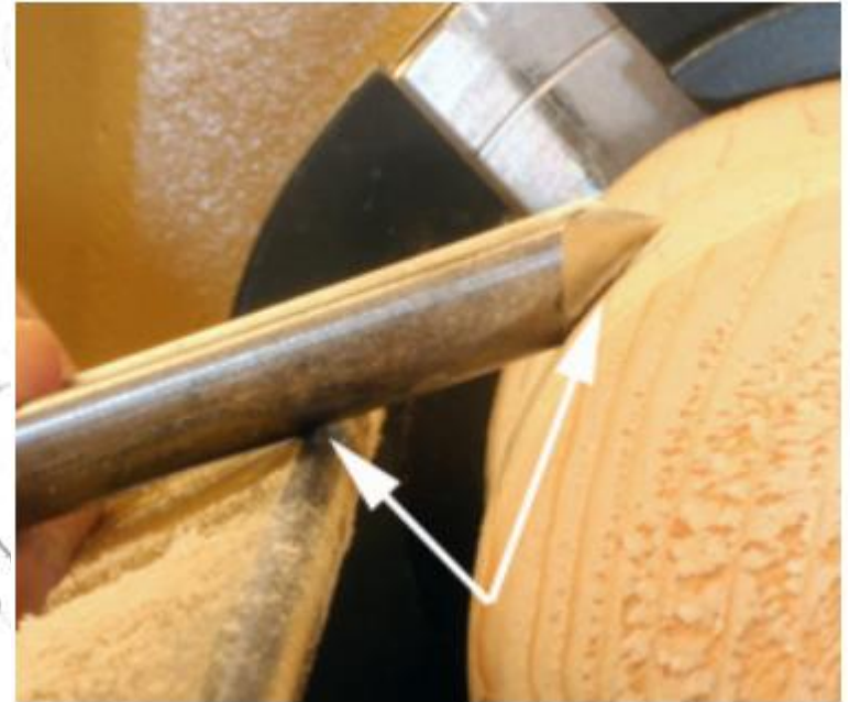
Fig 5.3a Safe angle of presentation, i.e. on the heel of the bevel
